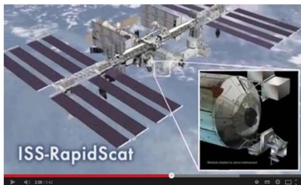
The upgrades began this month with the first NASA Earth-observing instrument to be mounted on the exterior of the space station: **ISS-RapidScat will monitor ocean winds for climate research, weather predictions and hurricane science.** The Cloud-Aerosol Transport System--"CATS" for short--a laser radar that can measure clouds along with airborne particles such as pollution, mineral dust, and smoke. **CATS will follow ISS-RapidScat on another SpaceX flight targeted for December.**
