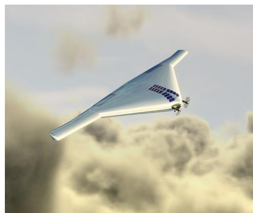
One possibility for sampling the clouds of Venus on the drawing boards is the Venus Atmospheric Manoeuvrable Platform (VAMP). It flies like a plane but floats like a blimp. It could stay aloft in Venus' cloud layer for up to a year gathering data and samples.
