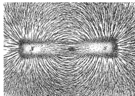
Lines of force shown with a magnet and iron filings via Physics Stack Exchange
