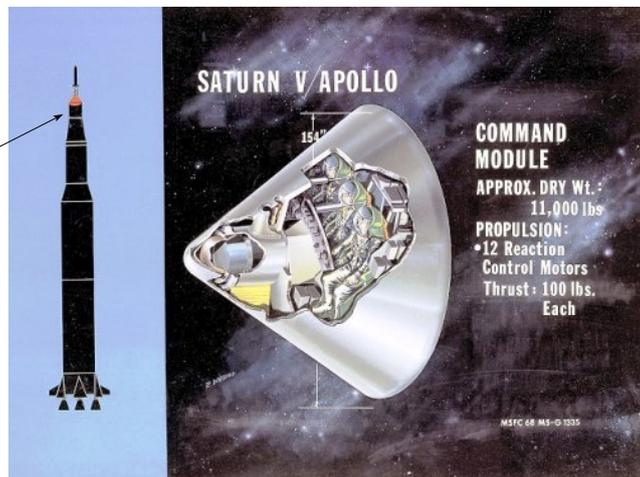
Apollo 11 left Earth via a type of rocket now no longer used, called a Saturn V. The rocket was 111 metres tall, about the height of a 36-story-tall building.
