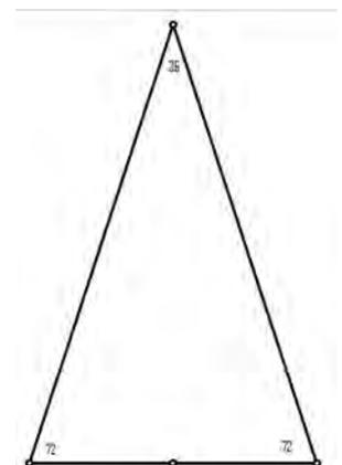
The Golden Triangle, with the apex angle =  $36^\circ$  and the two base angles =  $72^\circ$
