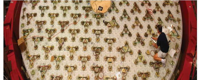
Hundreds of actuators will constantly adjust the mirrors to counteract atmospheric turbulence measured by laser pointer.
